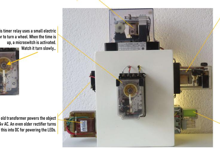
This timer relay uses mechanical friction to implement switching slowly. You can see its internals move when activated.
