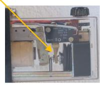
This is an old 24v AC relay that takes care of switching between the two timers. Because it's so big you can easily see it switch.
